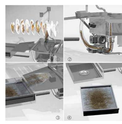
$\ensuremath{\textbf{Phase}}\xspace$  0: Coarse soiling is removed from the wash ware early, in the pre-wash zone.
